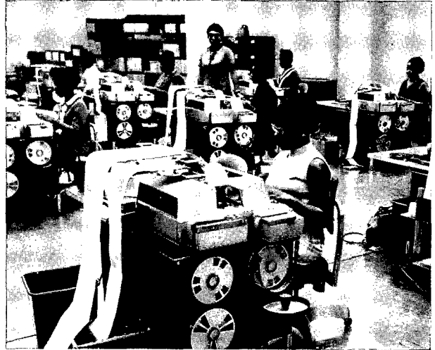
Automatic writing machines being used to process immigrant visas at the Central Office. An eight-channel punched paper tape is produced that can be rerun on auxiliary equipment using various program tapes to produce other required forms to provide evidence of alien registration and gather statistical data.
